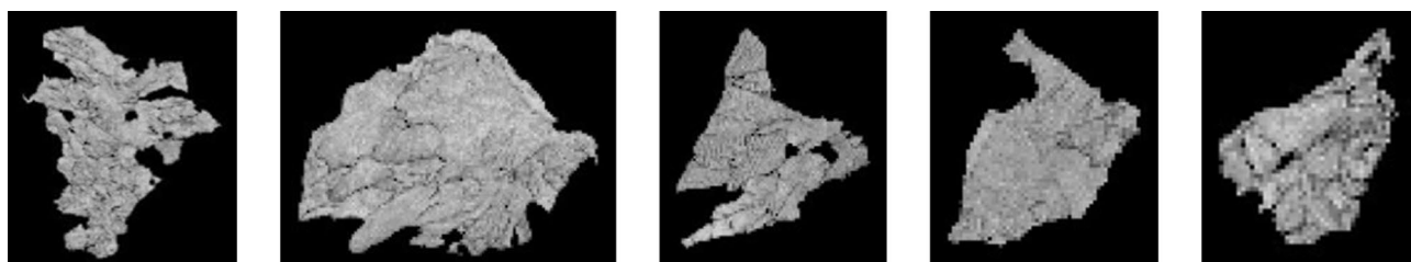
Figure 4. Examples of segmented EBSD images by grain (Steel D). Pixel size of the leftmost image is 90 by 86.
