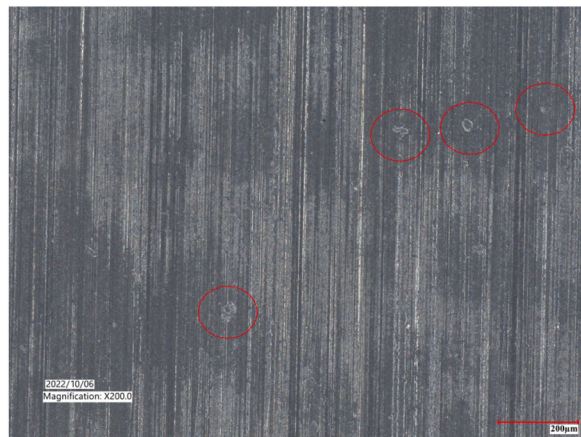
Fig. 12. Image of grind damage on nonirradiated sample.
