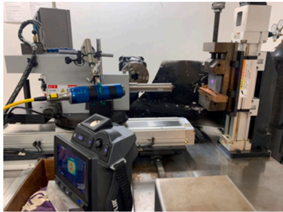
Fig. 2. Laser & thermal camera set up.
