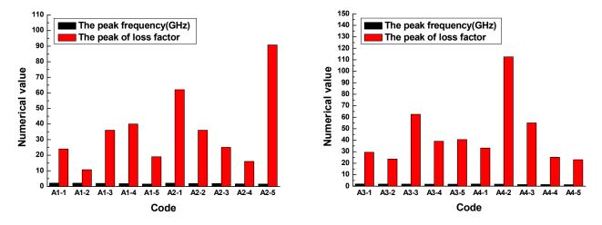
Figure 12. The peak and peak frequency of the loss factor of the rubber samples.
