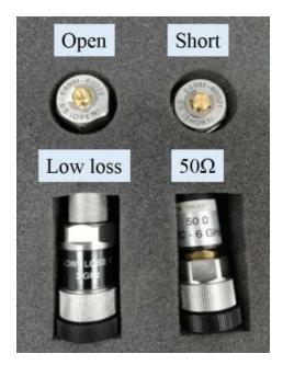
Figure 2. Four standard parts for calibration.
