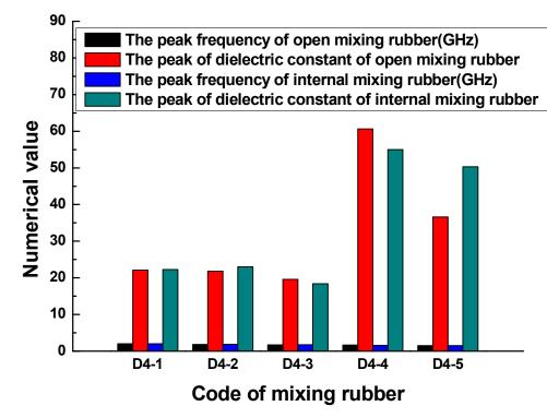
Figure 6. The peaks of the dielectric constant and frequency of the rubber samples.
