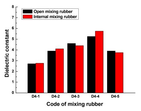
**Figure 8.** The maximum dielectric constants of the rubber samples obtained by different mixing processes.
