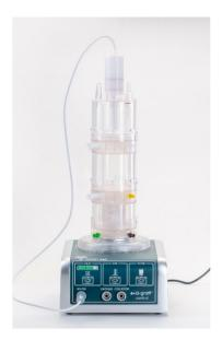
**Figure 2.** Separation system for regenerative cells from adipose tissue Q-graft<sup>®</sup> (Human Med AG, Schwerin, Germany) consisting of the disposable part Q-graft<sup>®</sup> collector (top) and the reusable control unit Q-graft<sup>®</sup> control (bottom).
