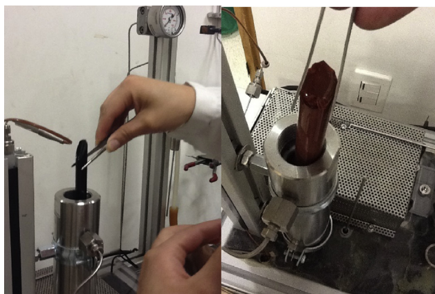
Fig. 1. Polymeric gel when introduced to the supercritical drying reactor for sample Ae25 and Ae200.
