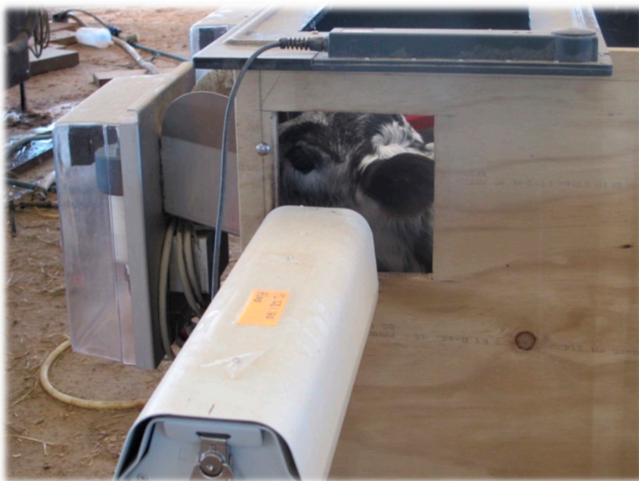
Figure 9. Infrared thermography (IRT) camera installed on the left side of the automated calf feeder collecting thermal infrared images of the facial region through the square viewing hole as a calf feeds from the feeder.
