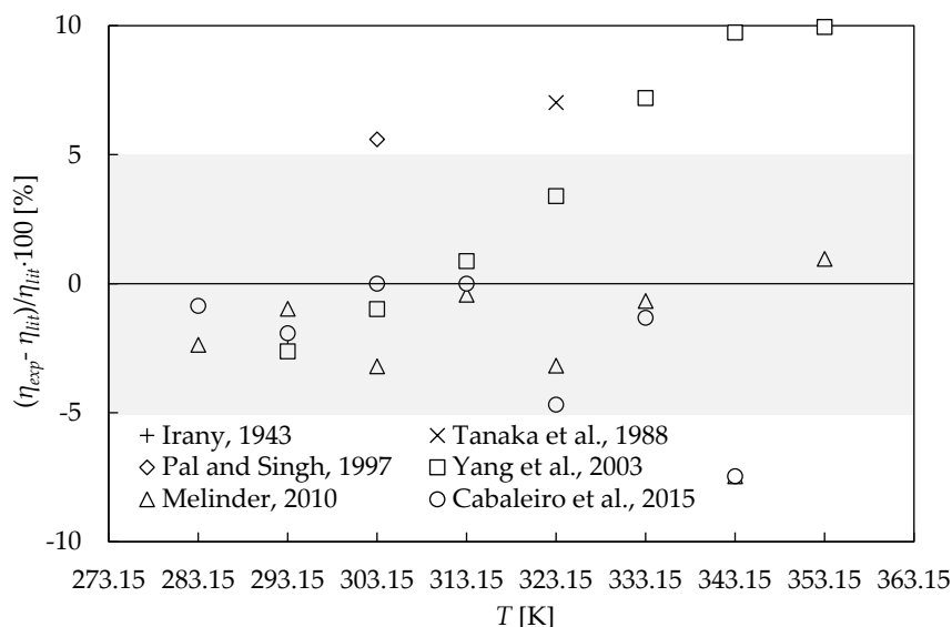
Figure 2. Percentage relative deviations among the experimental dynamic viscosities ( \eta_{\text{exp}} ) and literature values ( \eta_{\text{lit}} ) [42–47] for the ethylene glycol:water mixture 50:50 vol%. The grey area represents the declared expanded uncertainty ( k = 2 ) region of the rheometer, 5.0%.
