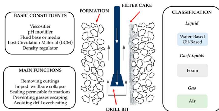
**Figure 1.** Schematic of the drilling operation, including main constituents, main function, and classification of drilling fluid. Reprinted with permission from Zamora-Ledezma et al.<sup>5</sup> Copyright 2022 ACS Publications.
