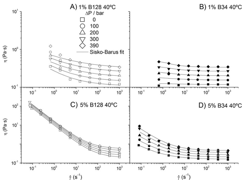
**Figure 2.** Experimental viscous flow curves and Sisko–Barus model fitting for the different OMMT/oil fluids studied as a function of pressure at 40 °C: (A) viscous flow curve for the lowest B128 concentration, (B) viscous flow curve for the lowest B34 concentration, (C) viscous flow curve for the highest B128 concentration, and (D) viscous flow curve for the highest B34 concentration. Reprinted with permission from Hermoso et al.<sup>19</sup> Copyright 2014 Elsevier.
