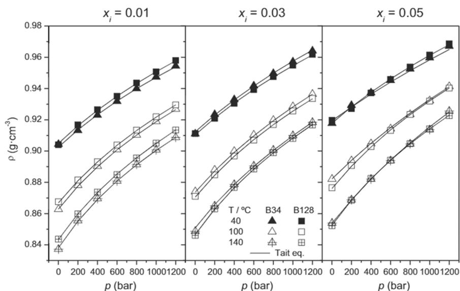
**Figure 3.** Evolution of the experimental density with pressure at different temperatures for OMMT/oil fluids. Reprinted with permission from Hermoso et al.<sup>71</sup> Copyright 2017 Elsevier.
