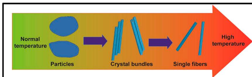
**Figure 6.** Organization change of OPAL in oil with the temperature rising. Reprinted with permission from Zhuang et al.<sup>79</sup> Copyright 2017 Elsevier.
