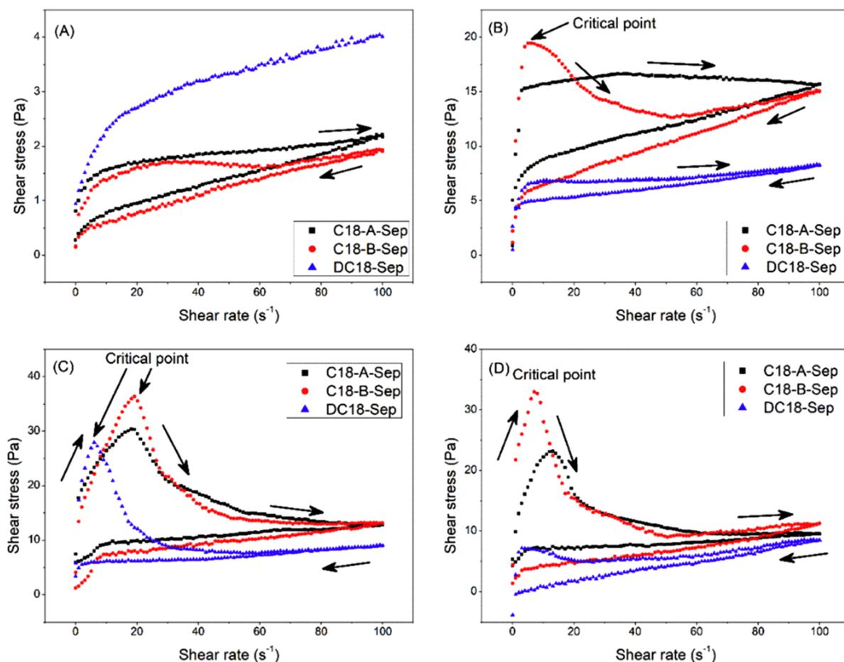
**Figure 7.** Dynamic rheological curves of OSEP/oil fluids aged at (A) 66 °C, (B) 150 °C, (C) 180 °C, and (D) 200 °C for 16 h. Reprinted with permission from Zhuang et al.<sup>87</sup> Copyright 2018 Elsevier.
