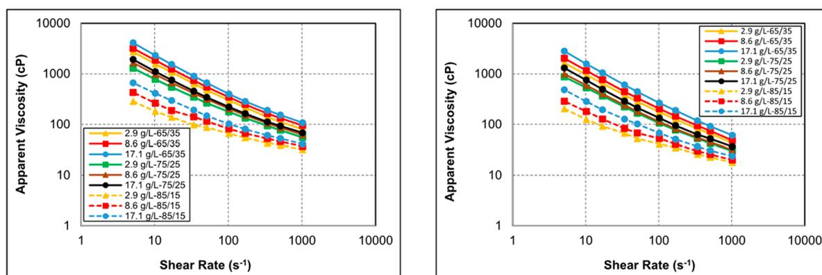
**Figure 8.** Effects of OC concentration and OWR on the apparent viscosity of the OBM at 52 °C (right) and 79 °C (left). Reprinted with permission from Fakoya and Ahmed.<sup>93</sup> Copyright 2018 Elsevier.
