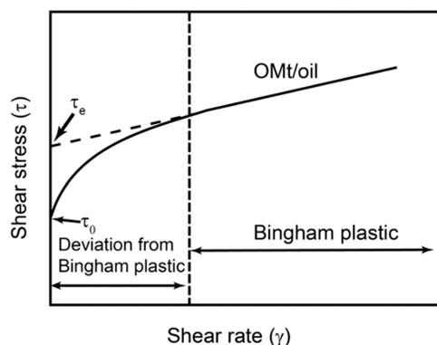
**Figure 4.** Interpretative diagram of the rheological model of the OMMT/oil fluid. Reprinted with permission from Zhuang et al.<sup>7</sup> Copyright 2016 Elsevier.
