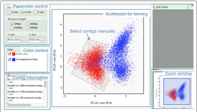
**Fig. 2** Graphical user interface of SAG-QC. Contigs are plotted as *dots* in the scatterplot based on sequence properties such as GC contents and k-mer frequencies. Users can enclose any regions manually and extract/remove contigs inside the region. Statistics of the enclosed contigs is in the "contig information" panel. Colors of the plots can be edited in the "color control" panel. Users can modify the parameters for drawing the scatterplot in the "parameter control" panel
