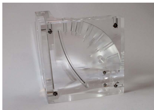
Fig. 6. Acrylic glass phantom holding two electrodes (one curved, one straight-line) equipped with titanium reference balls for accurate registration.
