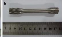
Figure 1 | Macrograph. (a), The bulk AlCoCrFeNi<sub>2.1</sub> EHEA ingot. (b), The tensile test specimen cut from the ingot.
