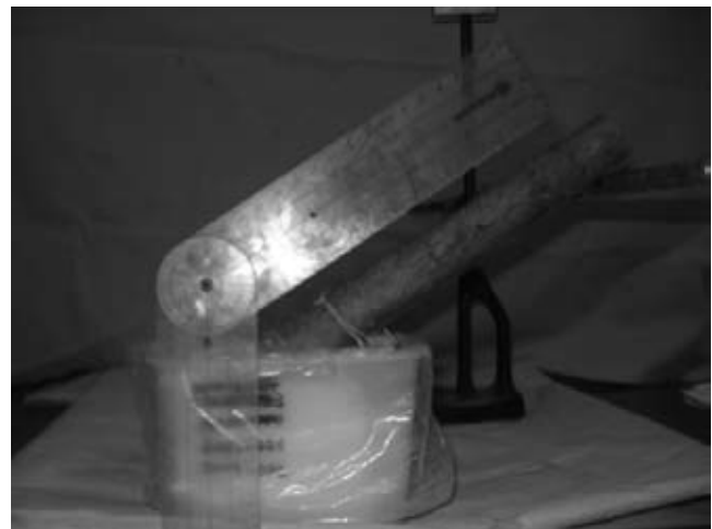
Figure 2. Vertical alignment of the femoral neck and cement fixation technique of the proximal femur.
