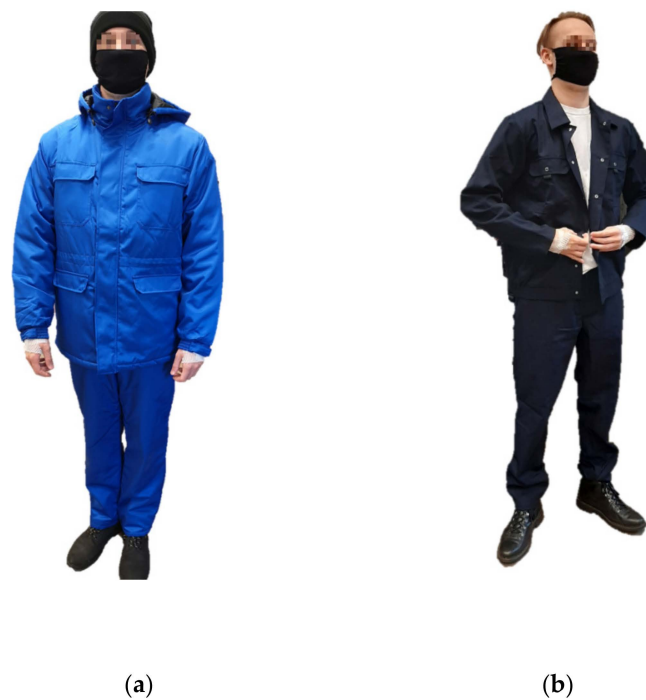
Figure 1. Photo of the clothing ensemble used in tests (from the left): (a) protective clothing for cold environment and (b) standard work clothing.
