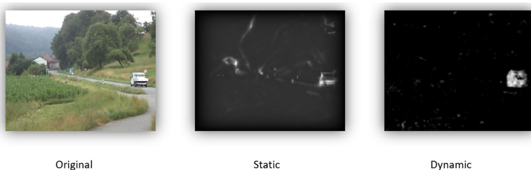
Fig. 1 Frame of a video stimulus ( left ) with corresponding static ( middle ) and dynamic ( right ) saliency maps calculated with TVSM. Contrasts and luminance influence the static map, while the moving truck in the otherwise steady scene dominates the dynamic saliency
