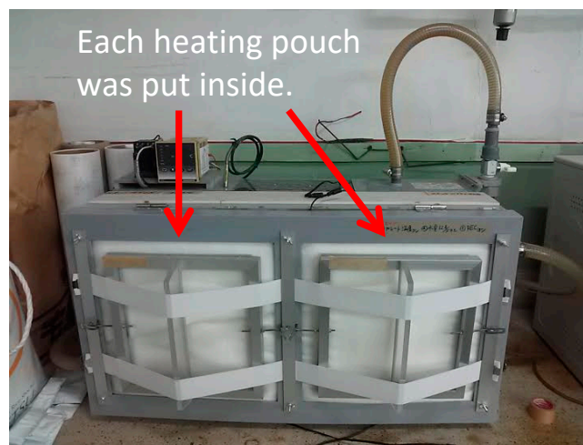
Figure 11. Temperature-measuring instrument. Each heating pouch was closely pressed against the temperature sensor plate inside the sealed box.
