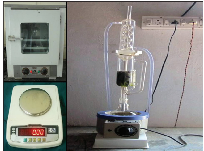
Figure 3: Armamentarium for plant extract apparatus -autoclave, weighing machine, soxhlet apparatus
