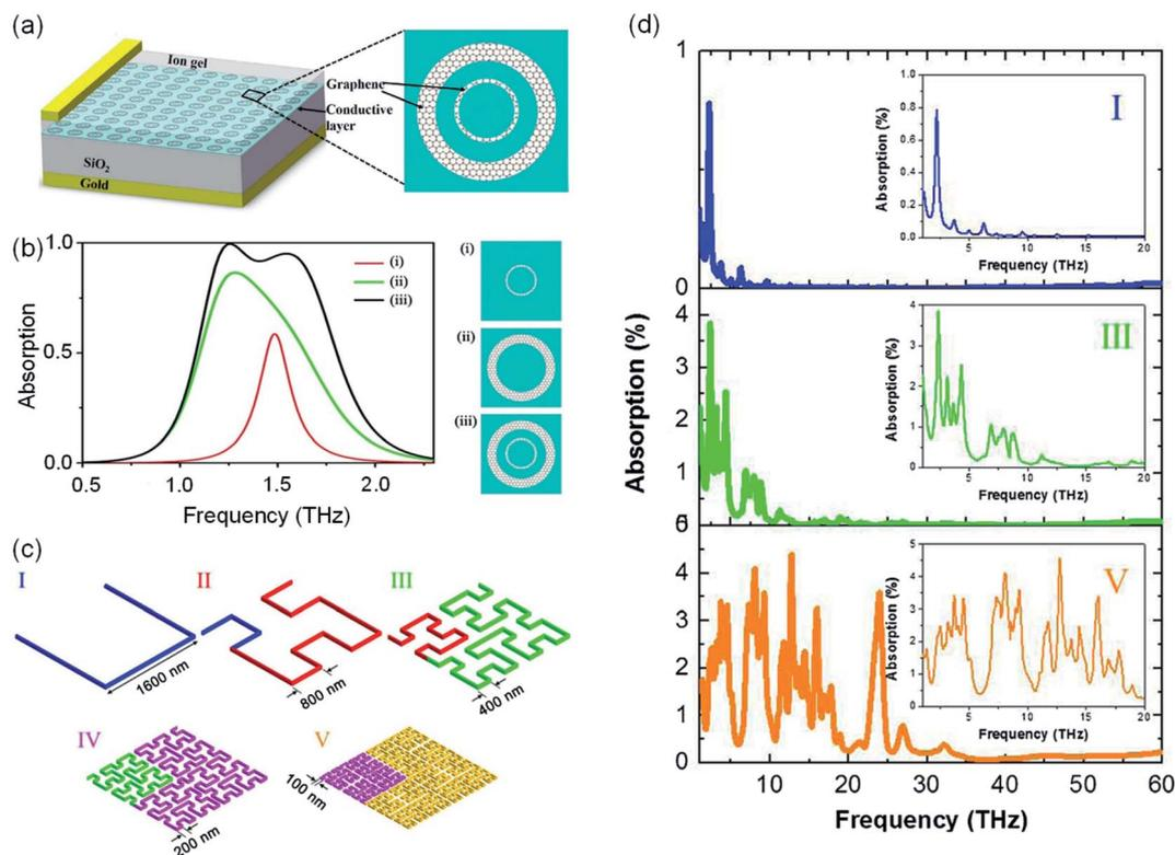
**Fig. 4** (a) Schematic of the THz absorber consisting of the GCDR. (b) Simulated absorptions of the proposed GCDR absorber with different graphene patterns (reproduced with permission from ref. 66 Copyright 2018 The Optical Society). (c) Iterative construction of the Hilbert curve for the first five (I–V) levels. (d) Simulated absorptions for graphene Hilbert structures of levels I, III, and V (reproduced with permission from ref. 69 Copyright 2016 American Physical Society).
