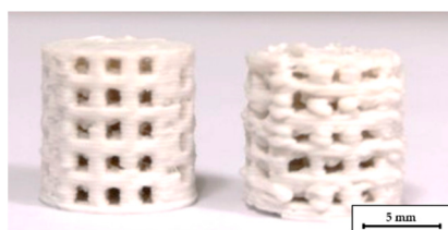
Figure 5. C2 based scaffolds printed at 205 °C, for the left one a 0.4 mm nozzle was used, for the right one a 0.5 mm nozzle.
