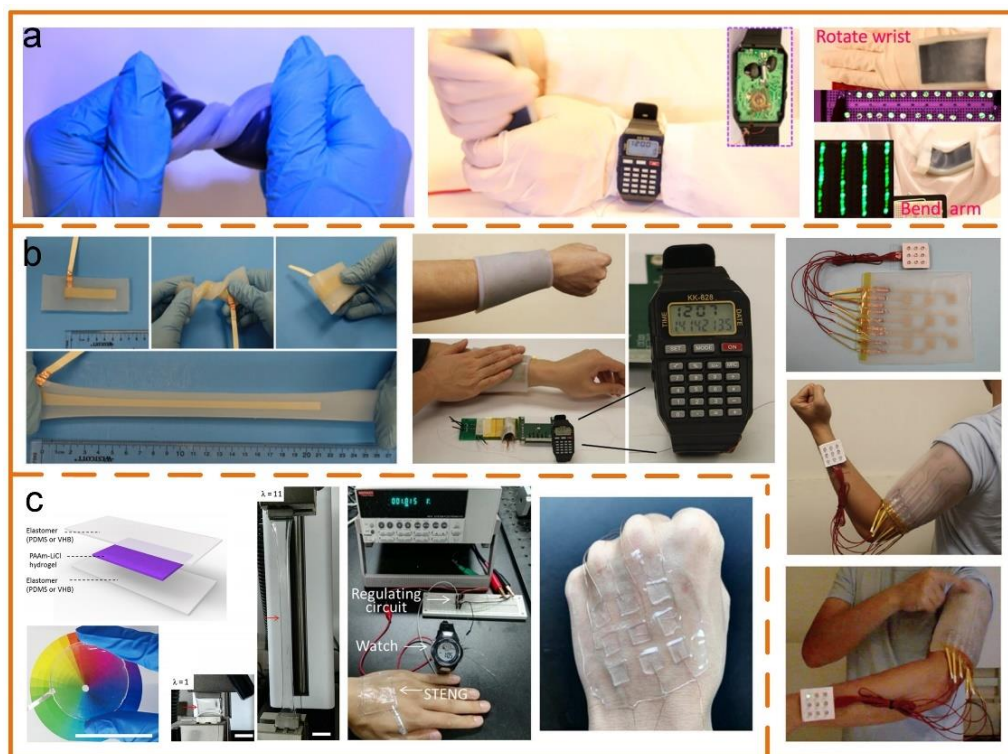
Figure 10. Self-powered sensors based on flexible and stretchable TENGs. (a) A stretchable and waterproof TENG based on carbon black electrode. Reproduced with permission [118]. Copyright 2016, American Chemical Society. (b) A super-stretchable NG based on Ag NWs electrode. Reproduced with permission [124]. Copyright 2016, John Wiley & Sons. (c) Ultrastretchable, transparent TENG based on PAAm-LiCl hydrogel electrode. Reproduced with permission [127]. Copyright 2017, American Association for the Advancement of Science.
