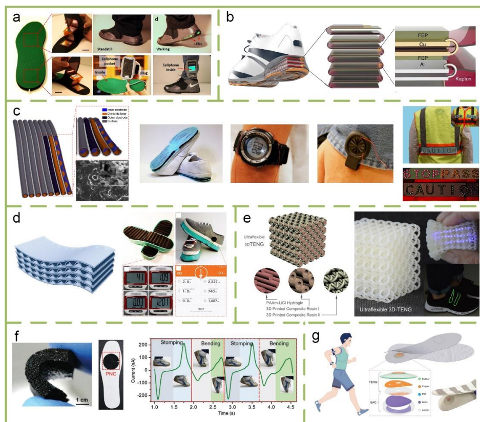
Figure 11. Smart shoes based on TENGs. (a) A packaged power-generating insole with built-in flexible multi-layered TENGs. Reproduced with permission [132]. Copyright 2013, Elsevier. (b) A multilayer TENG embedded into the sole to exploit human biomechanical energy. Reproduced with permission [133]. Copyright 2015, Springer Nature. (c) A soft TENG fabricated by elastomeric materials and a helix inner electrode sticking on a tube with the dielectric layer and outer electrode. Reproduced with permission [119]. Copyright 2016, Springer Nature. (d) A TENG with a multilayer elastomeric structure with closely stacked arches as basic functional units as a continuous energy source for wearable electronics. Reproduced with permission [120]. Copyright 2017, John Wiley & Sons. (e) A practical, ultraflexible, and three-dimensional TENG fabricated by 3D printing. Reproduced with permission [134]. Copyright 2018, Elsevier. (f) Stretchable porous carbon nanotube-elastomer hybrid nanocomposite for harvesting mechanical energy and detecting motion types. Reproduced with permission [135]. Copyright 2017, John Wiley & Sons. (g) A TENG-based smart insole for multifunctional gait monitoring. Reproduced with permission [136]. Copyright 2019, John Wiley & Sons.
