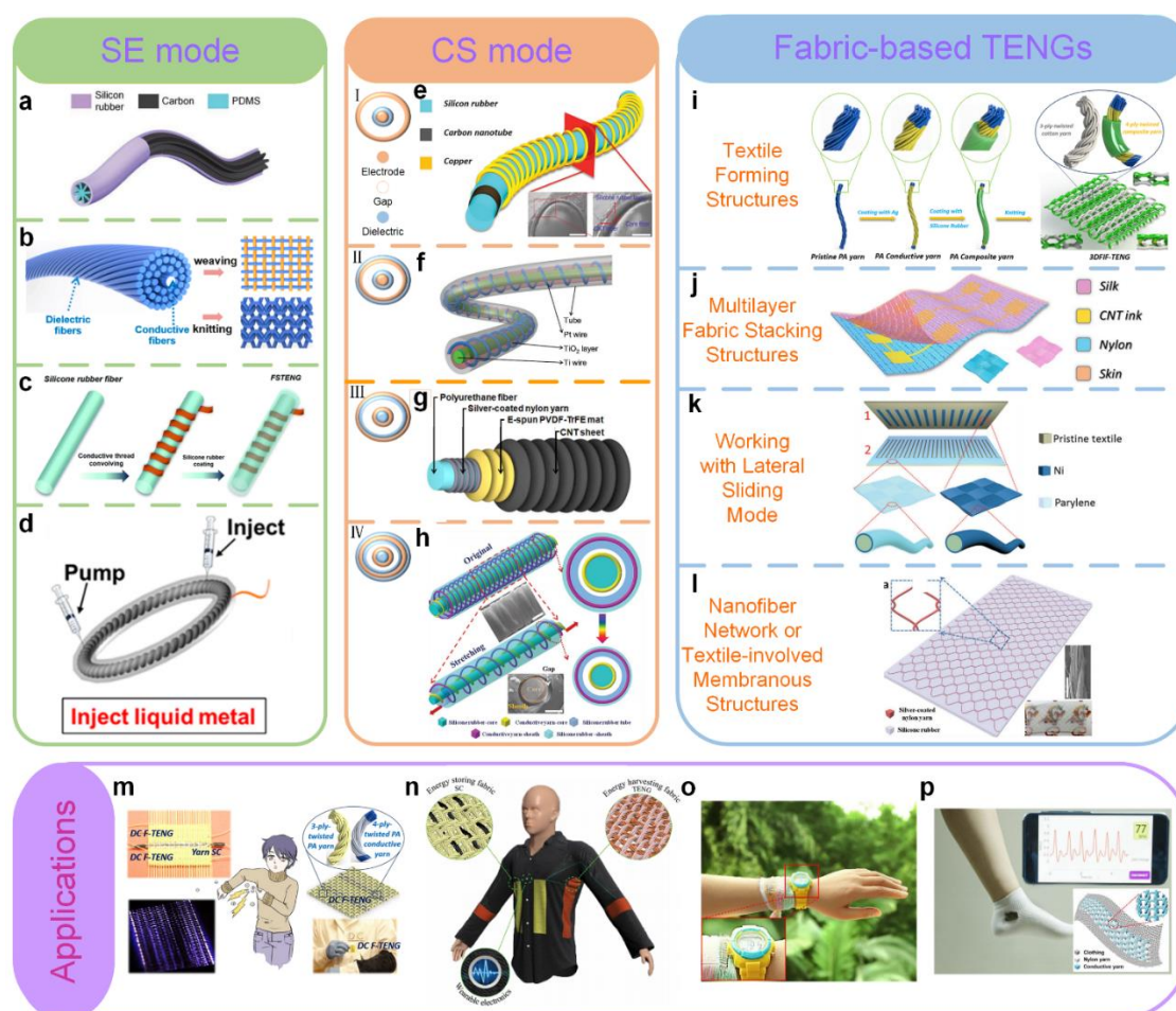
Figure 22. Fiber and fabric-based TENGs and some smart applications. (a) Typical design of dielectric polymers directly wrapped around core fiber electrodes to build SE mode fiber-based TENGs. Reproduced with permission [214]. Copyright 2018, John Wiley & Sons. (b) Typical design of tightly twining artificial fibers around a conductive core fiber to build SE mode fiber-based TENGs. Reproduced with permission [215]. Copyright 2017, American Chemical Society. (c) Typical design of twining fiber electrodes on the surface of stretchable fibers to build SE mode fiber-based TENGs. Reproduced with permission [216]. Copyright 2017, Royal Society of Chemistry. (d) Typical design of injecting nontoxic liquid metals into stretchable tubes to build SE mode fiber-based TENGs. Reproduced with permission [217]. Copyright 2014, American Chemical Society. (e) Typical design of type I (dielectric layer wrapped around inner electrode as the core and only outer electrode as the shell). Reproduced with permission [218]. Copyright 2017, John Wiley & Sons. (f) Typical design of type II (dielectric layer wrapped around an inner electrode as the core and the same configuration as the shell). Reproduced with permission [219]. Copyright 2016, John Wiley & Sons. (g) Typical design of type III (inner electrode wound on a dielectric fiber as the core and the same configuration as the shell). Reproduced with permission [220]. Copyright 2016, Springer Nature. (h) Typical design of type IV (the outer surface of the type III further covered by a dielectric or encapsulation layer). Reproduced with permission [221]. Copyright 2018, John Wiley & Sons. (i) Typical design of fabric-based TENGs with textile forming structures. Reproduced with permission [222]. Copyright 2020, Elsevier. (j) Typical design of fabric-based TENGs with multilayer fabric stacking structures. Reproduced with permission [157]. Copyright 2018, American Chemical Society. (k) Typical design of fabric-based TENGs working with lateral sliding mode. Reproduced with permission [219]. Copyright 2016, John Wiley & Sons. (l) Typical design of fabric-based TENGs with nanofiber reticular or textile-involved membranous structures. Reproduced with permission [223]. Copyright 2018, John Wiley & Sons.
