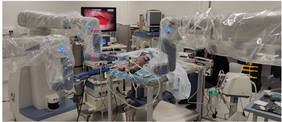
Fig. 1 Setup of the experiments. The Senhance can be seen with its three arms, operating a 10 mm camera and a 3 mm instrument in the right and left hand arm. An accessory video screen for the 2D display of the operating field is on the left side. In the background, the Draeger Primus is positioned for anesthesia
