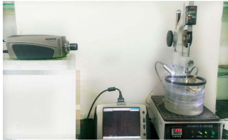
Figure 2. The penetration test process recorded by the high-speed camera.
