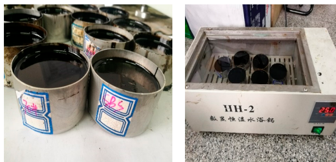
Figure 1. Asphalt samples and the process of the water bath.
