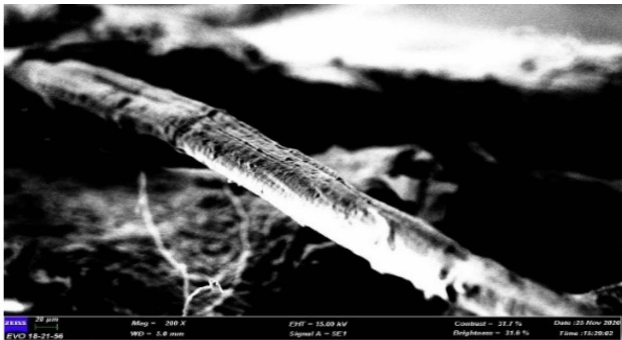
Figure 8. SEM micrograph of banana leaf fibre.
