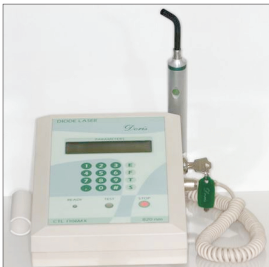
Figure 2. Laser device used in the study. A gallium aluminum arsenide diode laser (CTL-1106MX; Doris, Warsaw, Poland) with 820 nm wavelength was used.
