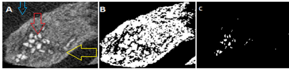
Figure 11. Axial view of micro-CT indicates an area of bone formation which appears gray (yellow arrow), the surrounding soft tissue appears black (blue arrow) and area of the remaining cement in white color (red arrow). B: Binary picture of the threshold of the same image. C: The white particles of the remaining cement analyzed by Sky scan image analysis software. doi:10.1371/journal.pone.0107403.g011
