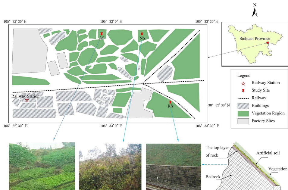
Figure 1. Detailed locations of the study sites. Notes: RS = railway slope; NS = a naturally developed slope within 1 km of the railway; AS = an agricultural slope within 1 km of the railway. This map was generated by the authors by using the ArcGIS (version 10.0). The photographs in this map was taken by one of the authors (Shunan Chen).
