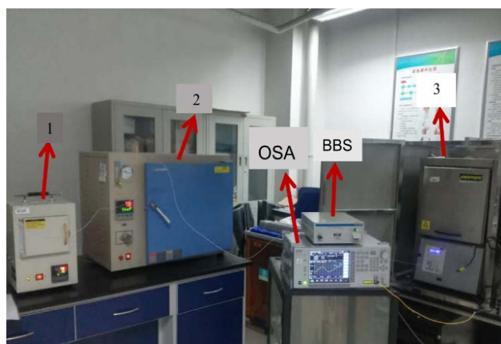
Figure 5. The experimental site of the multipoint temperature sensing system. The light from the broad-band light source (BBS) emits into the cascaded MZIs, and the MZIs are placed in three furnaces, respectively. The final superposition of the three sensors is obtained through the optical spectrum analyzer (OSA).
