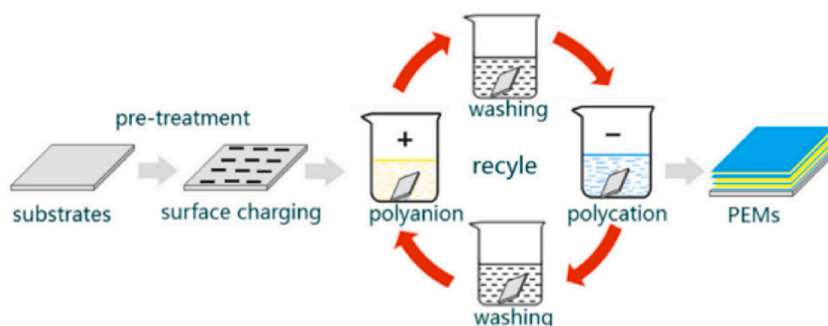
Fig. 10. A schematic representation of the LbL assembly process. Reproduced from Ref. [14] with permission.
