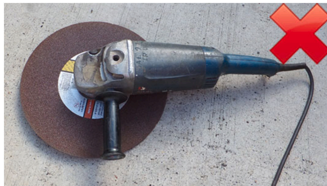
Fig. 1. Angle grinder with protective guard removed to fit a larger disc. https://www.worksafe.qld.gov.au/injury-prevention-safety/alerts/whsq/2017/guards-and-discs-on-angle-grinders .
