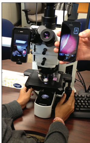
Figure 5: Live video transmission of a digital image is shown from a cell phone attached to a microscope with the Magnifi adapter
