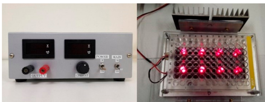
Figure 10. Our own designed NIR-PIT illuminator was constructed by 8 light-emitting diodes (LED: SMBB690D-1100-02 \times 8, EPITEX, Inc., Kyoto, Japan), whose peak wavelength of emission is 690 nm. The power density of the LEDs is controllable from 0 to 600 mA (0–244.86 mW/cm 2 ).
