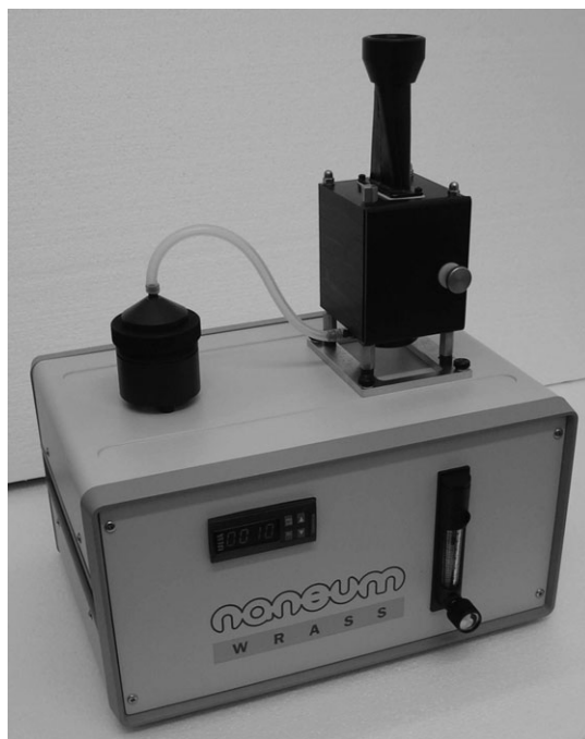
Fig. 11. A WRAS aerosol sampling system with a timer on the left of the front panel, a needle valve to control the flow rate (on the right of the front panel) and a digital flow indicator (on the top).
