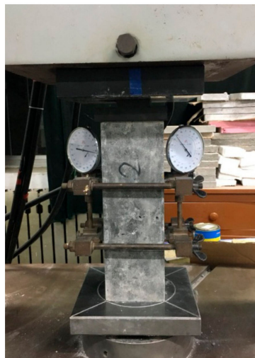
Figure 2. Test setup of elastic modulus.
