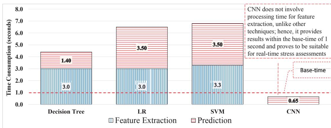
Figure 10. Performance comparison in terms of assessment time for real-time applications.
