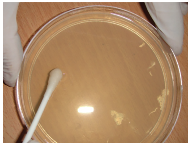
Fig. 3: Swab sample smeared on the SDA plate
