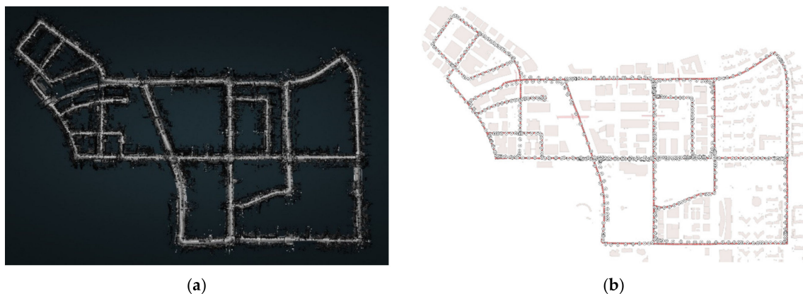
Figure 8. Top view of the test site in Pangyo, South Korea. (a) Collected point cloud data [32], (b) Distribution of observation positions.
