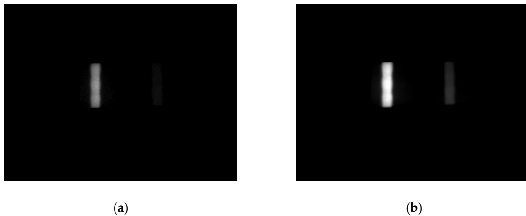
Figure 7. Detection result of a low-concentration strip: (a) original image; (b) after range adjustment.
