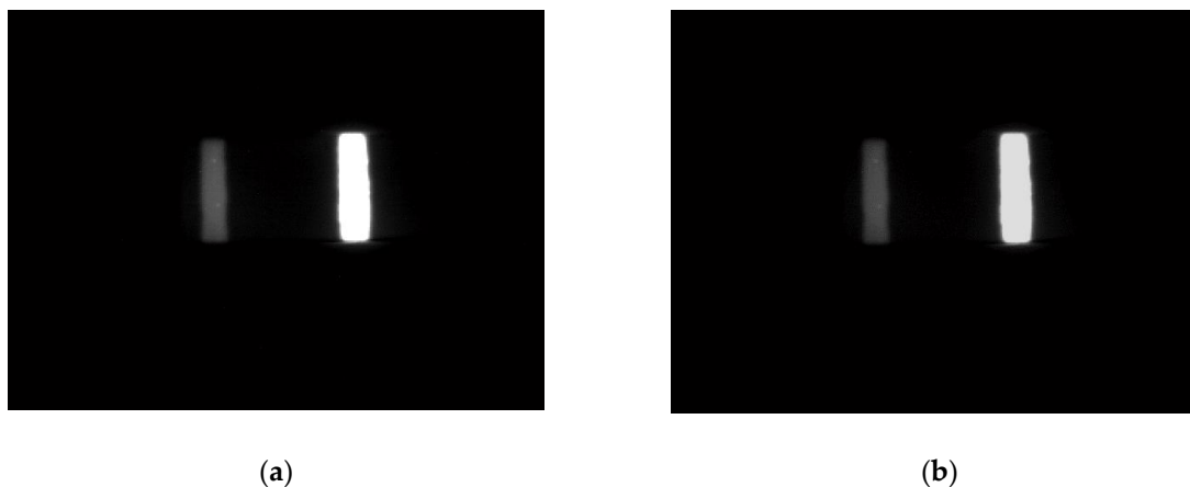
Figure 8. Detection result of a high-concentration strip: (a) original image; (b) after range adjustment.
