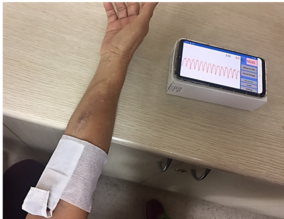
Figure 3. The hemodialysis patient during testing using a pulse radar sensor. Note that the App displays the signal waveform on a mobile phone. The detailed strategy of immobilizing as developed by the VWM monitoring system on patients, shown in Appendix A.
