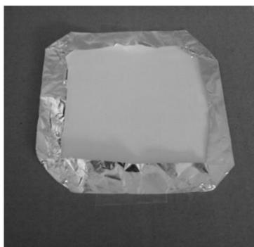
Figure 1. Example of a paper patch with the aluminium foil backing.
