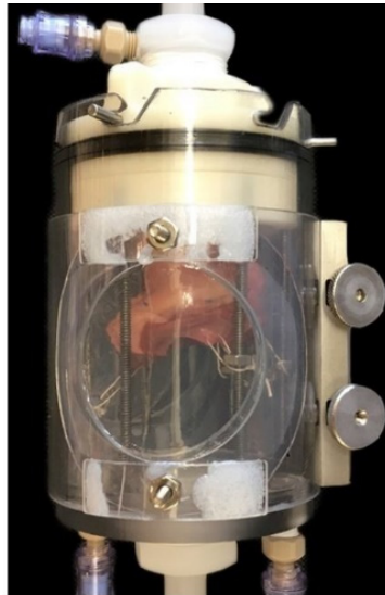
Figure 4. Actual photograph of porcine valve suspended in the valve chamber.
