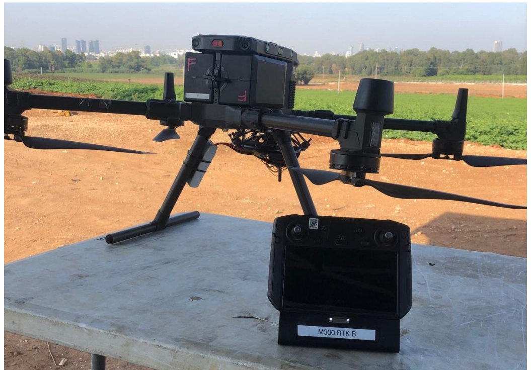
Figure 6. DJI Matrice 300 RTK used in the field experiments.
