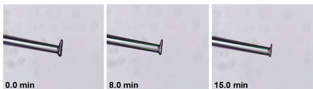
Figure 10. Images of an ibuprofen particle at different time points (0.0, 8.0 and 15.0 min) during an on-going dissolution measurement in the micropipette-assisted microscopy technique.
