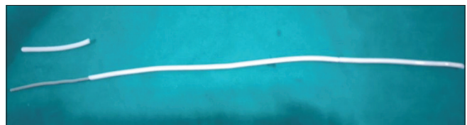
Figure 1: Broken plastic sleeve of the stylet
