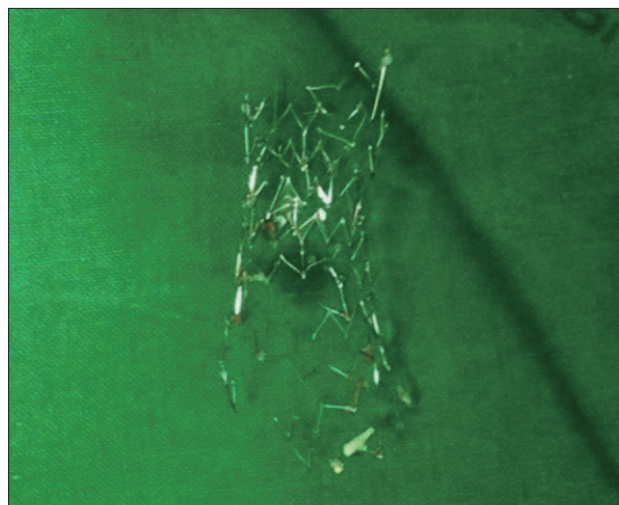
Fig. 3. The stent strut which retrieved by open heart surgery.
