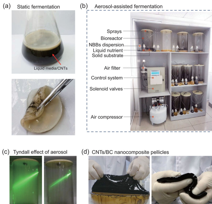
Figure 2. Comparison between traditional static fermentation and aerosol-assisted biosynthesis. (a) Static fermentation in the liquid nutrient dispersed with CNTs. The static fermentation in the liquid media failed to produce CNT/BC nanocomposite. (b) Experimental apparatus. Air is compressed by the air compressor and flows through the air filter to remove microorganisms. The liquid nutrients or NBB suspension are siphoned to the sprays and atomized into aerosol droplets with the compressed and filtered air, which is controlled by the solenoid valves and operated by the control system. (c) Tyndall effect of the aerosol. The Tyndall effect was observed after the spray of liquid nutrients and NBB suspension. (d) Photographs of CNT/BC nanocomposite pellicles. Uniform CNT/BC nanocomposite pellicle could be harvested directly from the solid substrate and the biosynthesized CNT/BC nanocomposites are flexible and mechanically robust.
