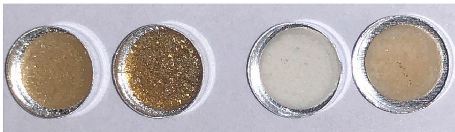
**Fig. 2.** Photographs of the DSC pans containing the mixtures (from left to right) PVPVA64/HPC-SSL, PVPVA64/HPC-UL, HPMCAS-M/HPC-SSL and HPMCAS-M/HPC-UL taken after the DSC runs.
