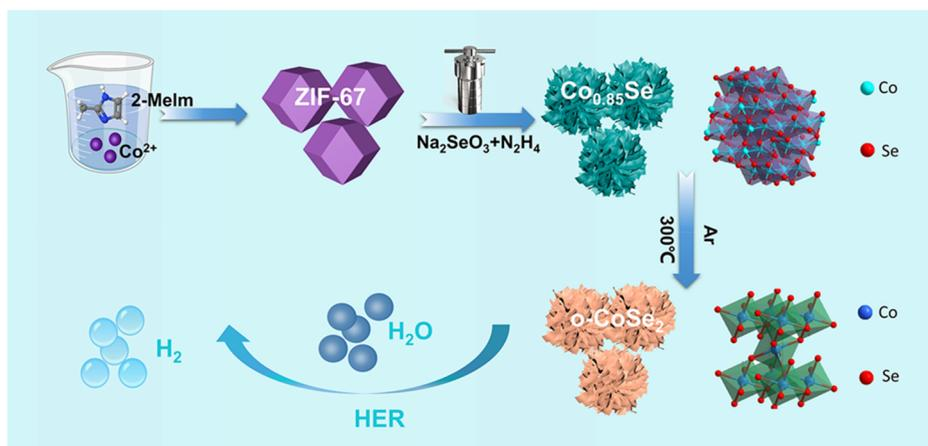
**Figure 1.** Schematic illustration of o-CoSe<sub>2</sub> NNS derived from Co<sub>0.85</sub>Se NNS for the alkaline HER.
