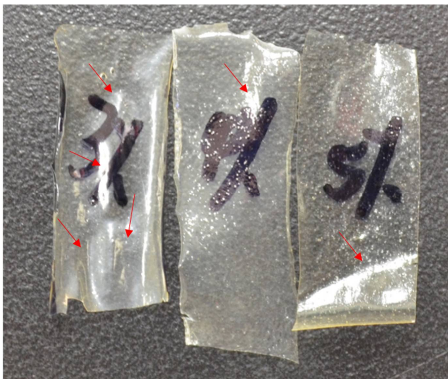
Figure 9. Picture for chitosan films after they were crosslinked and dried. The red arrows point to the wrinkles on the film.
