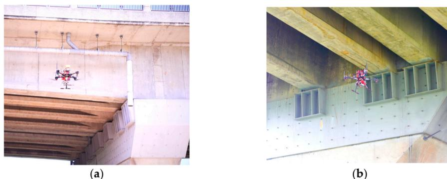
**Figure 14.** Bridge inspections performed by the self-assembled UAV: (a) operation on the side of the Wuling Bridge; (b) operation at the bottom of the Wuling Bridge.
