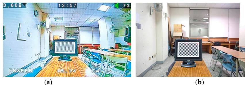
**Figure 3.** Camera's field of view and lens distortion. (a) original UAV camera image (b) inspection camera image.
