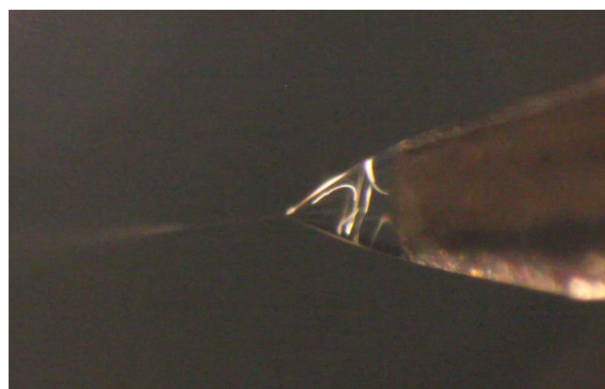
Fig. 6. Photograph showing the appearance of bubbles from the ESI capillary. The ESI is at near room temperature while the column is kept at 100°C. The cavitation stops when the ambient around the ESI emitter is pressurized to >1 atm.
