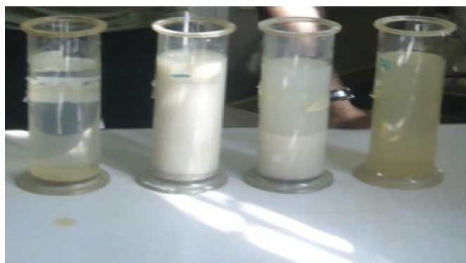
Figure 2. View of conducting a double Hydrometer Test on dispersive soil.
